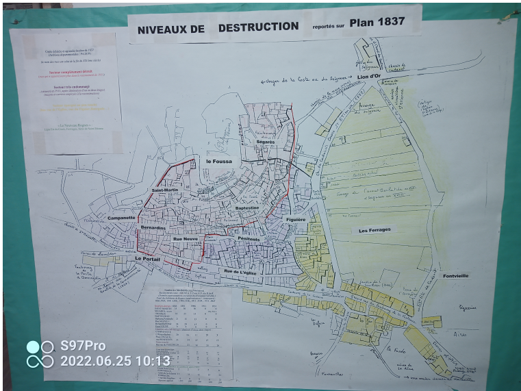
Figure 9: Distribution of the damage during the 1909 earthquake reported on a map of 1837. Red: destroyed. Purple: highly damaged. Yellow: Slightly damage. Green: rebuilt district after the 1909 earthquake. Source: "Les Amis du Patrimoine de Rognes", archives départementales: P4 2819.
