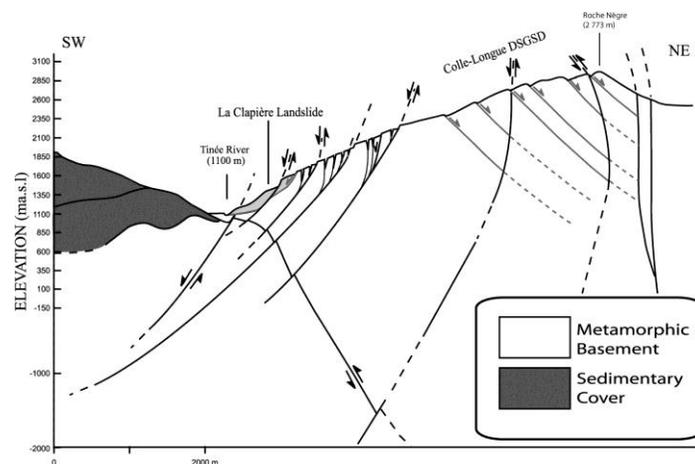
Figure 24 : cross section through the La Clapière slope (Jomard et al., 2014)
