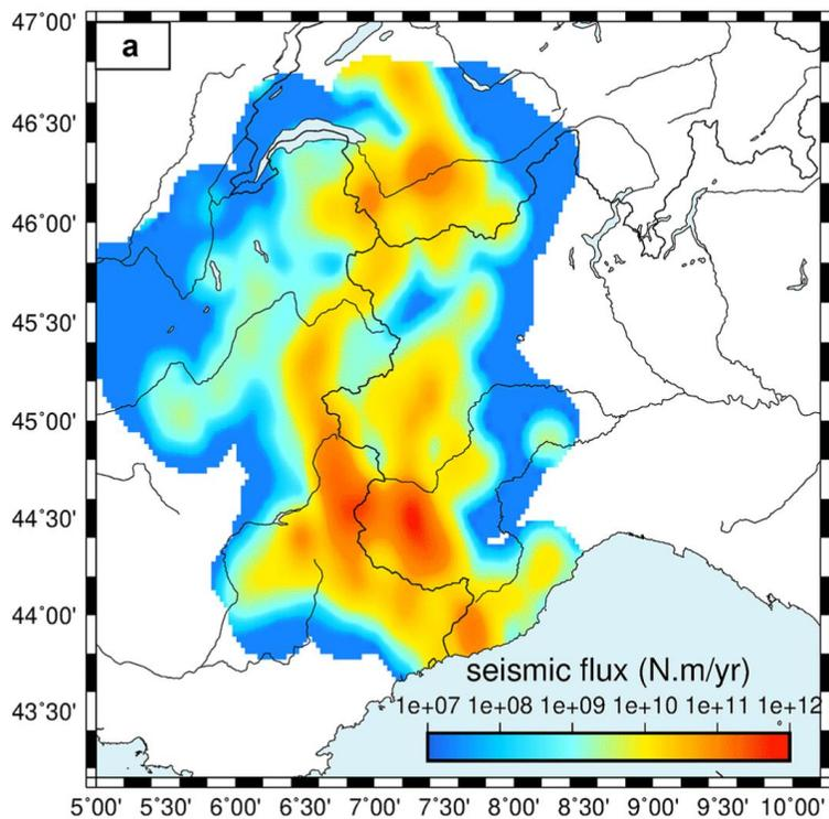
Figure 38 : Smoothed seismic flux over the western Alps (computed using annualized seismic moment for the period 1989 – 2014; Mathey et al., 2021)
