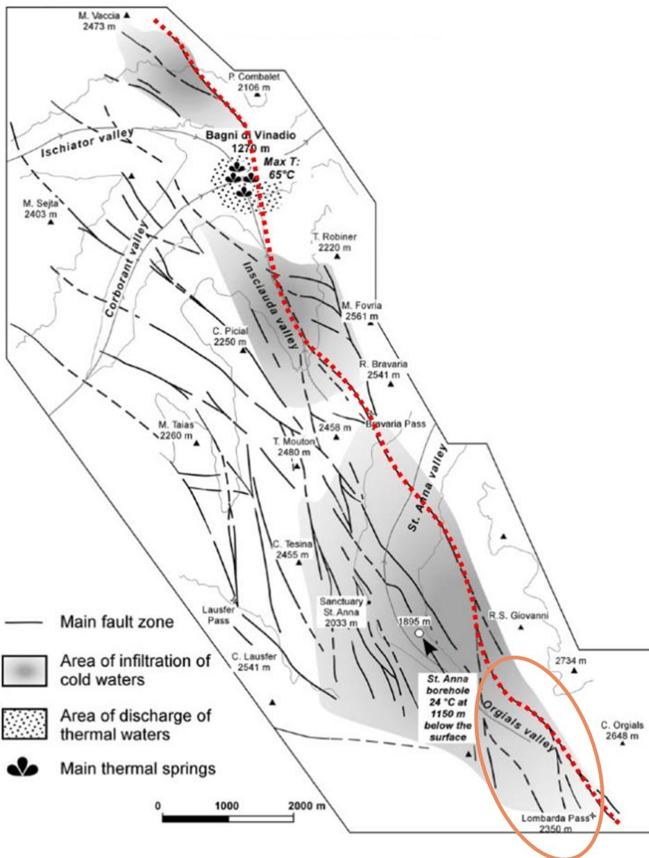
Figure 32 : Detailed map of faults around the principal Bersezio fault system (red dots) north of the Orgials valley (orange circle); greyish zones represent areas of cold water infiltration, drained in faults and flowing as hot springs in Bagni di Vinadio (Tmax: 65°C) – Adapted from Baietto et al., 2009
