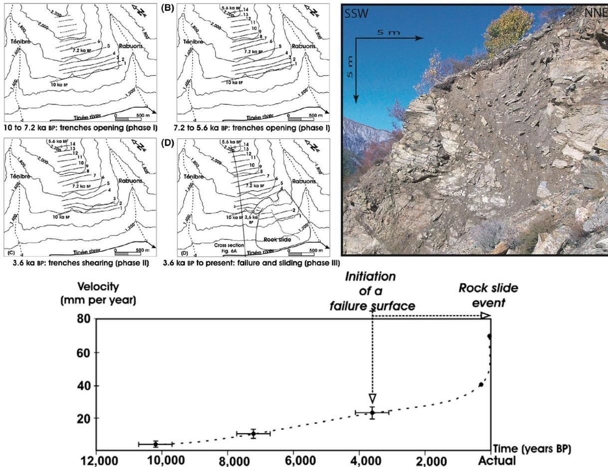
Figure 23 : evolution of the La Clapière slope inferred through morphological mapping and cosmogenic nuclide dating. View of an opened trench in cross-section (adapted from El Bedoui et al., 2009 and Jomard et al., 2014)
