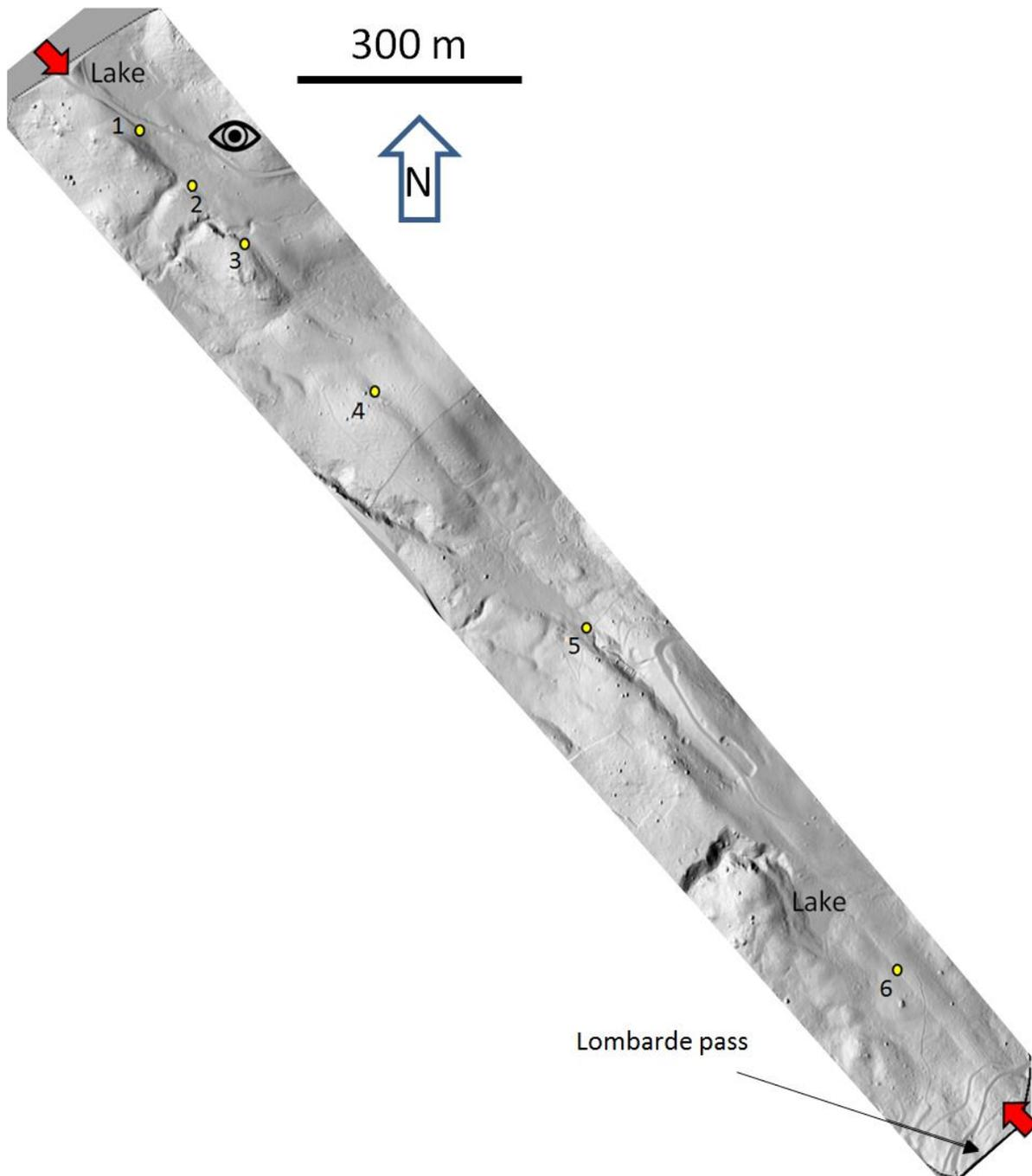
Figure 29 : Drone DEM of the 2km length Bersezio fault segment, and location of points of interest 1 to 6 (Vassallo et al., 2022)
