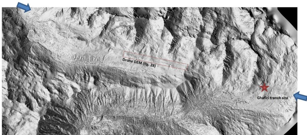
Figure 28 : Photogrammetric DEM derived from 1968 air photo. With the fault axis (blue arrows), location of high resolution drone DEM (red) and location of trenches dug by Ghafiri (1995, red star)
