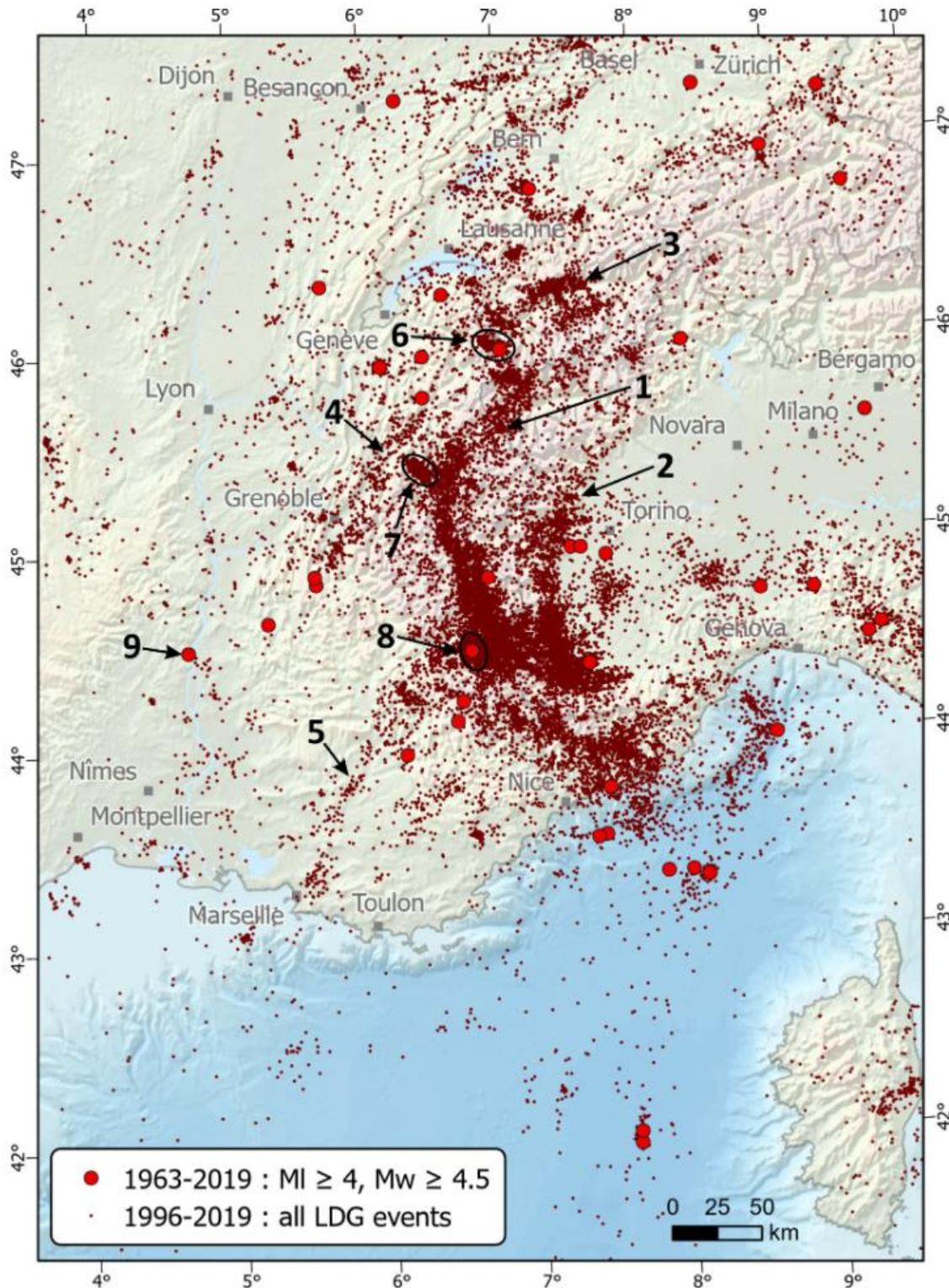
Figure 39 : Seismicity map from the CEA\_1996-2019 catalog supplemented by earthquakes of  $M_L \geq 4.5$  or  $M_w \geq 4.0$  from the CEA and the Si-Hex catalogs for the period 1963-1996. 1, 2: Briançonnais and Piemontais seismicity arcs respectively; 3-5: Rhône, Belledonne and Durance seismic alignments respectively; 6: Vallorcine cluster; 7: Maurienne cluster; 8: Ubaye cluster; 9: Epicenter of the Le Teil earthquake ( $M_w$  4.9, 2019/11/11). From Larroque et al., 2021.
