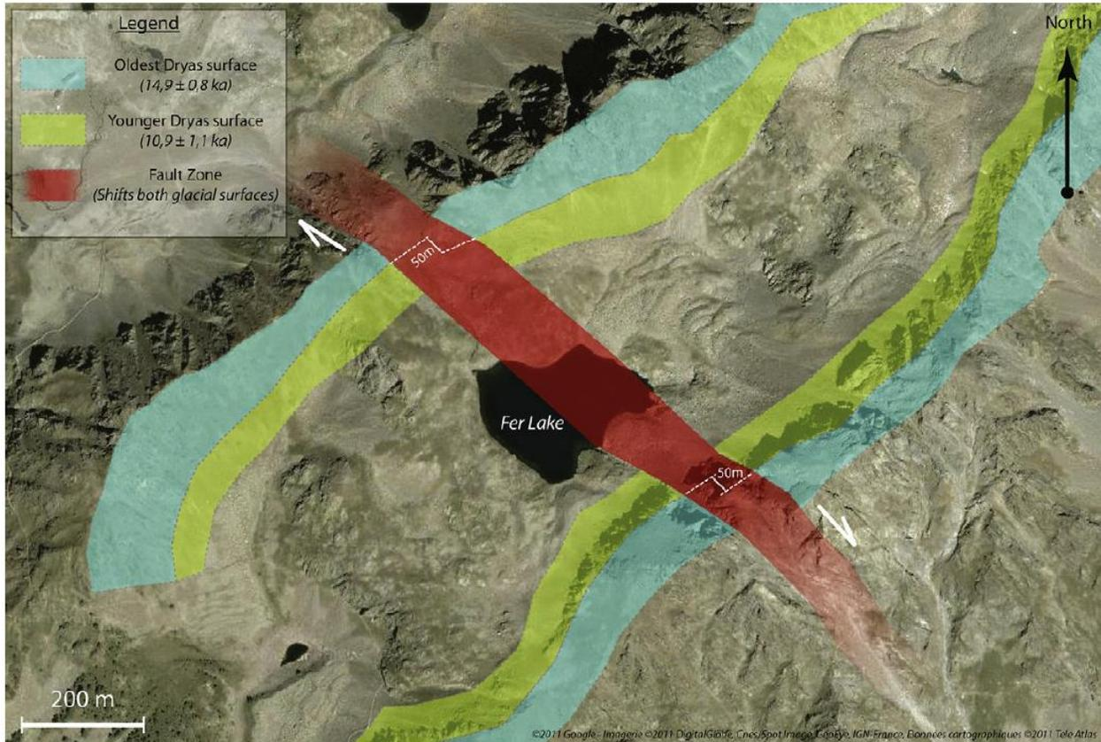
Figure 26: Right-lateral motion along a fault, interpreted as possible marker of Holocene active faulting occurring in between 10,9ky and 7,9 ky (Darnault et al., 2012)
