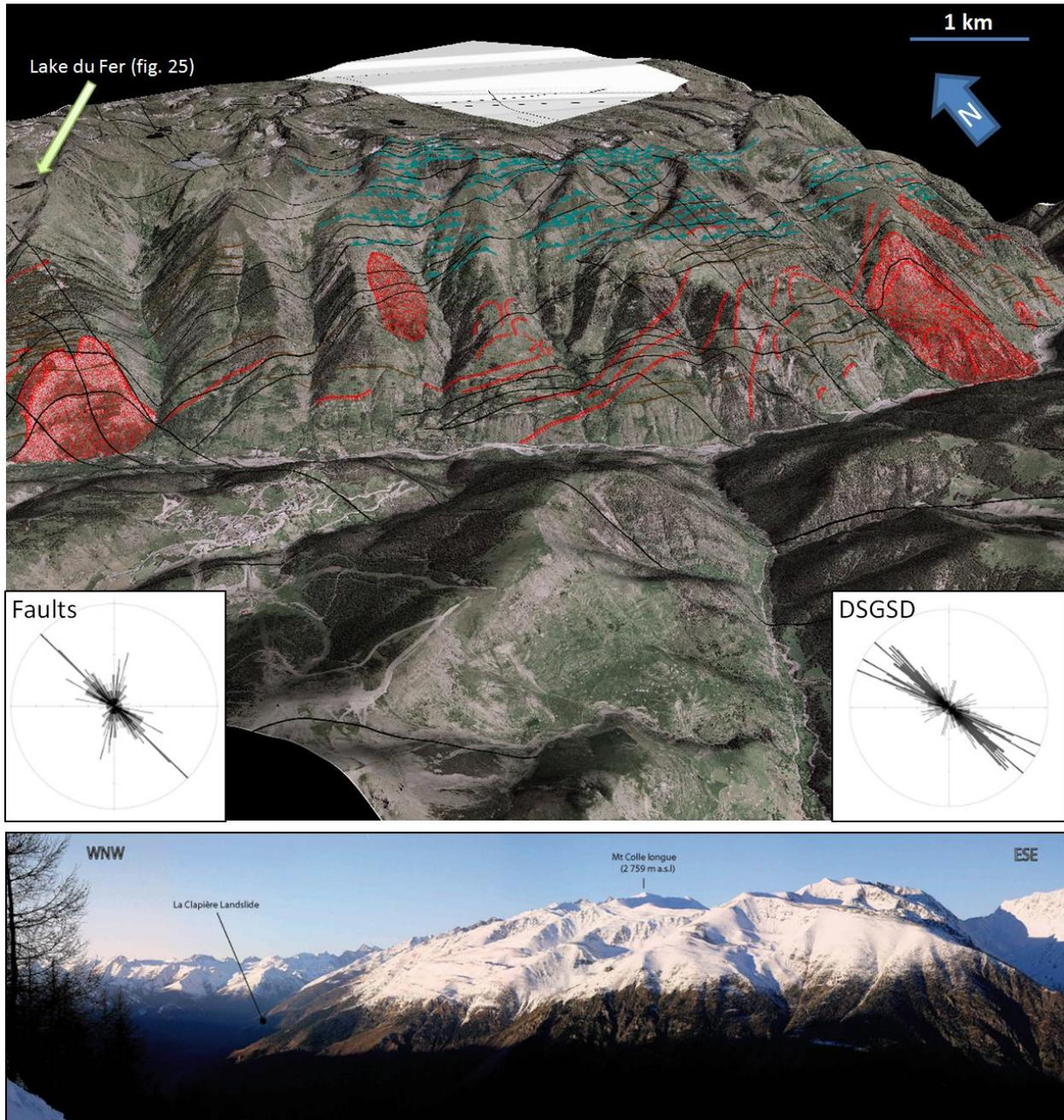
Figure 25 : Oblique 3D view over the Colle-Longue DSGSD and La Clapière with counterscarps (in green), scarps (in red), trenches (in brown) and faults (in black). Stereograms represent field measurements along faults and DSGSD morphologies (adapted from Jomard et al., 2014)
