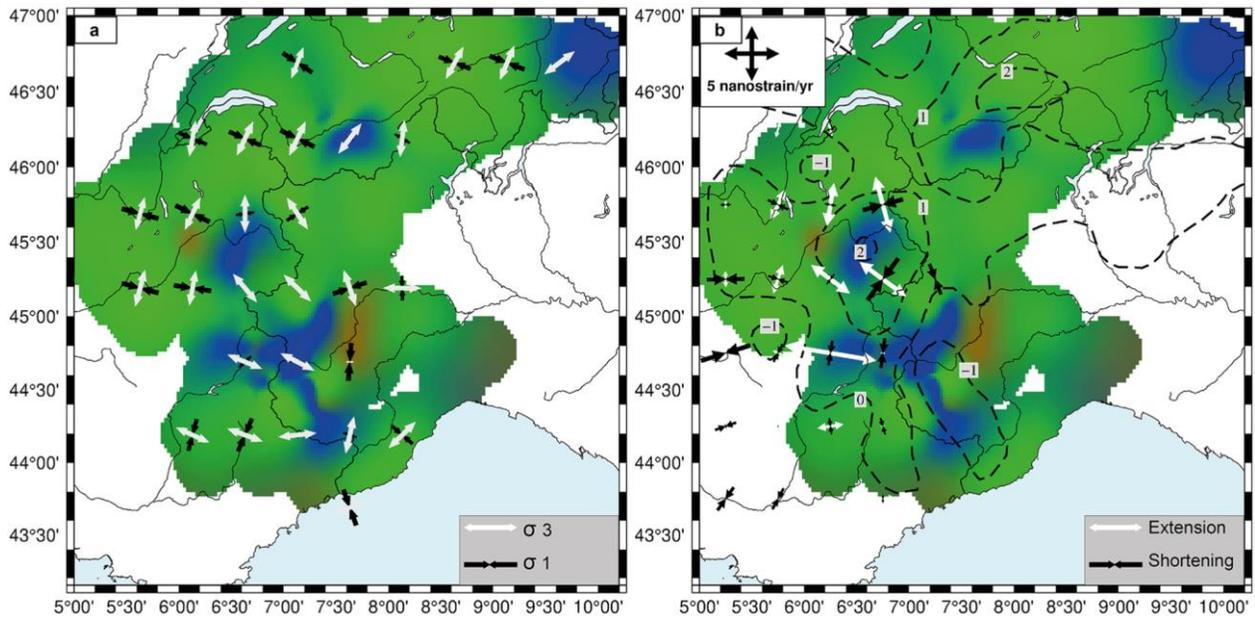
Figure 37 : Left: Stress orientation using focal mechanisms and smoothed interpolation (in red : compression, in blue : extension, in green : strike slip), Right: GNSS strain rates from Walpersdorf et al. (2018). Dashed lines represent contours of vertical velocities (in  $\text{mm yr}^{-1}$ ) from Sternai et al. (2019). Figures from Mathey et al., 2021
